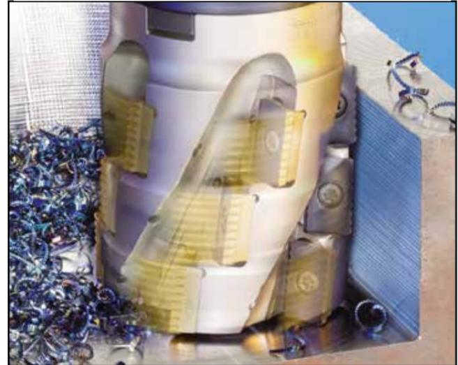
The MILLSHRED P290 line features 90° serrated or ribbed milling inserts. The serrations reduce the cutting forces, which make the cutters extremely productive at high overhangs.
