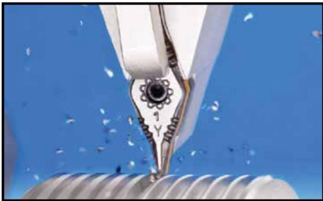
Iscar has added a clever new geometry to its line of small economical inserts. The new insert features a 25° corner angle, making it very cool for machining very narrow V-shaped grooves which cannot be machined by the standard insert.
