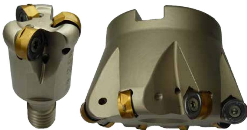
The H400 series from Iscar features round inserts with a very clever radius application -**like dropping a V8 engine into a cutter**. Unlike regular round inserts, the HELIDO 400 inserts have a periphery that consists of bounding arcs with radii that would only be found on round inserts twice their diameter.
