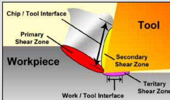
**This illustration shows the action that occurs in the cutting zone. Plastic deformation allows the chip to shear from the parent material in the primary zone.**
