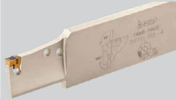
Rigid clamping in a tangentially oriented pocket. Tools available from 25mm to 500mm diameter range in 3mm to 4mm width. Tool holders available are either single or double ended blades. Machine at very high feed rates and interrupted cuts, and you still get an excellent surface finish.
