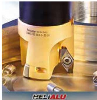
However, the characteristics of aluminium mean it's not always that simple. Aluminium exhibits high thermal conductivity and therefore the chips produced when machining transfer high levels of generated heat, resulting in significantly-reduced thermal loading of the cutting edge. Due to these properties, milling aluminium is characterised by extremely high cutting speeds and feeds.
